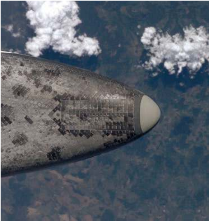
Space shuttle ceramic heat protection shield
